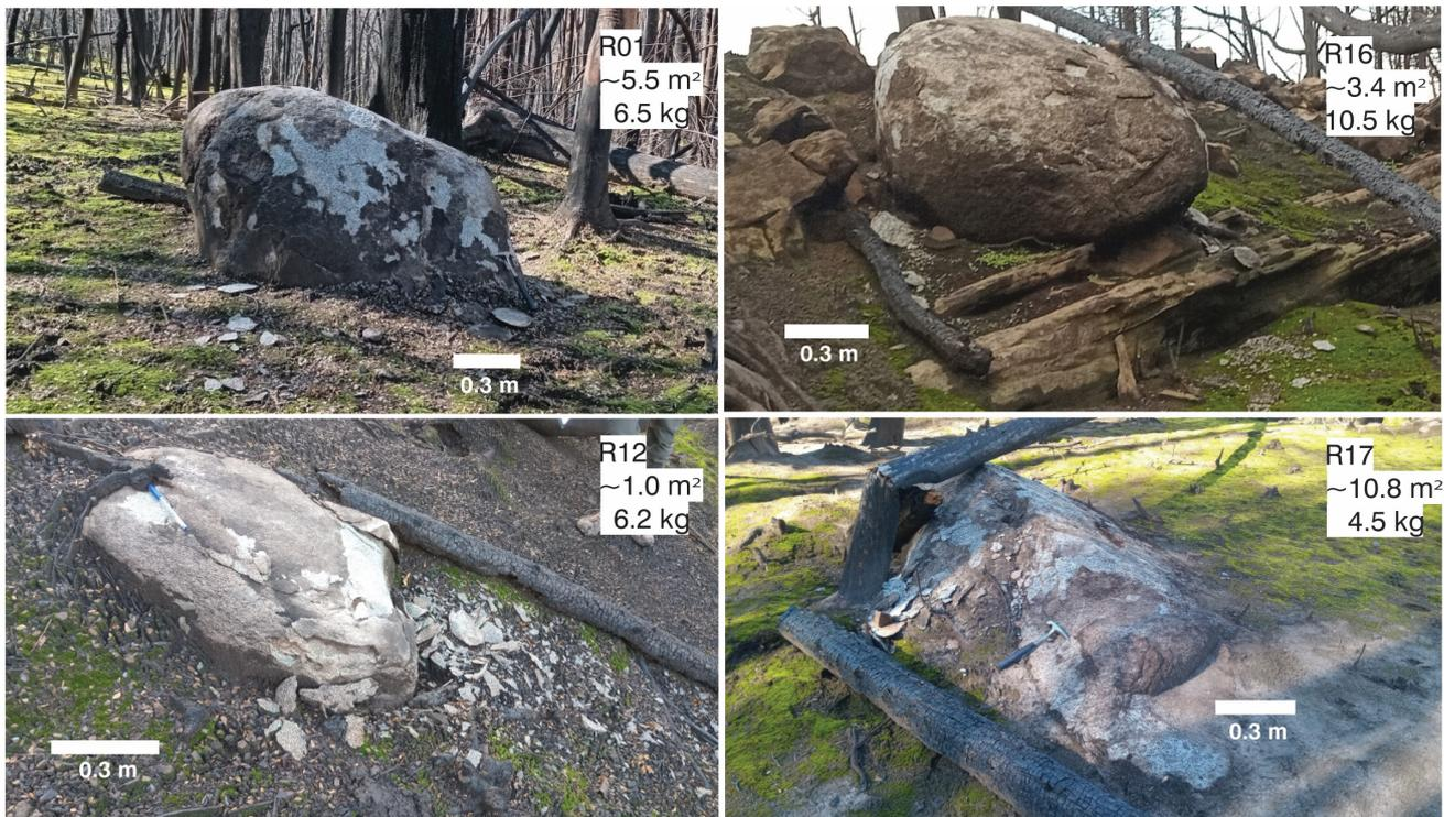
**Figure 1.** Granitoid erratic blocks surveyed after the LMRAFR fire (refer to fig. 2 for location details), with information provided for each block, including the estimated surface area and the total weight of sediment spalled by fire.
